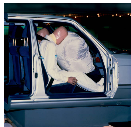
Figure 2.38 The car was originally travelling at high speed. When it hits the wall the car stops but the passenger stays in the original high speed state of motion. This results in the crash dummy hitting the steering wheel and the windshield (which is why it is a good idea to have safety belts and air bags).
